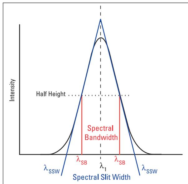
Figure 1: Gaussian intensity distribution of wavelengths emerging from the monochromator. The spectral bandwidth is defined by the red boundaries and  $\lambda_{SB}$ . The spectral slit width is depicted by the blue boundaries and  $\lambda_{SSW}$ .
