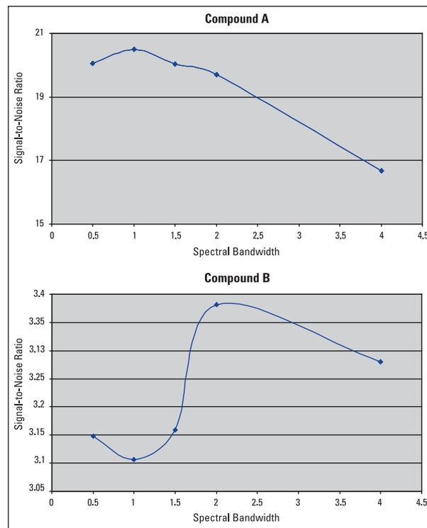
Figure 2: Graphical display of signal-to-noise ratio vs. spectral bandwidth for Compounds A and B. The maximum of the plot for Compound A indicates the maximum SNR occurs at a spectral bandwidth of 1.0 nm. The maximum of the plot for Compound B indicates the maximum SNR occurs at a spectral bandwidth of 2.0 nm.
